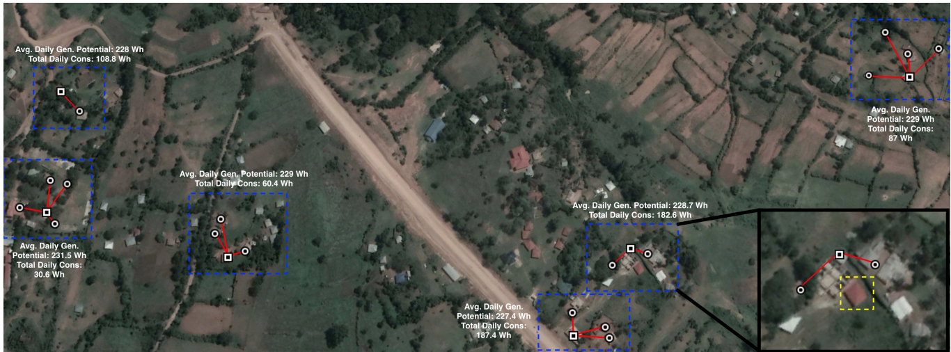
Figure 3: Layout of a scenario for energy sharing using star topology in one of the regions of Homa Bay County, Kenya. Each blue box shows the connections accomplished for each SHS in the area and its respective average daily energy generation potential and consumption. Squares illustrate SHSs and circles passive nodes. The yellow box shows an example household candidate that is not networked given the conditions of losses or load.
