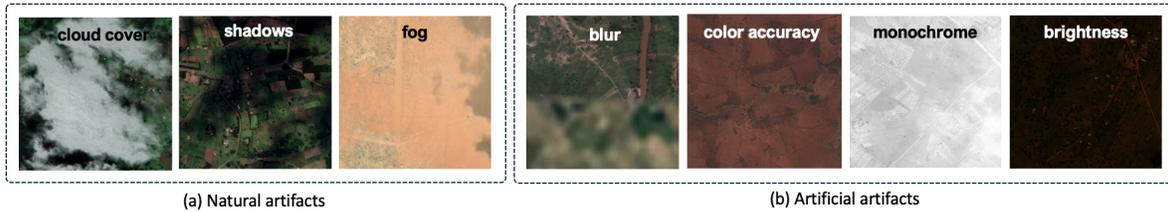
**Figure 1: (a) Natural artifacts during the image capture: undesired and inherent image phenomena were identified during the data collection step such as cloud cover, shadows produced by clouds, and fog due to sand in desert areas. (b) Examples of artificial artifacts encountered in the imagery collected using our data collection tool.**
